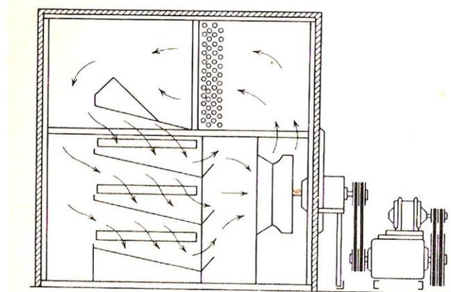
**Fig.3.Throughcirculation Tray drier**
