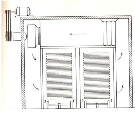
**Fig 1. Typical Tray Drier**
