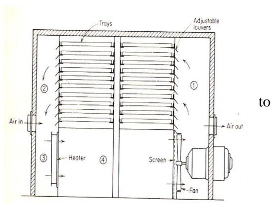
**Direct driers:** The construction of such driers depends greatly upon the nature of the substance being dried. Tray driers, also called cabinet, compartment, or shelf driers, are used for drying solids which must be supported on trays. This may include pasty materials such as wet filter cakes from filter presses, lumpy solids which must be spread upon trays, and similar materials. A
