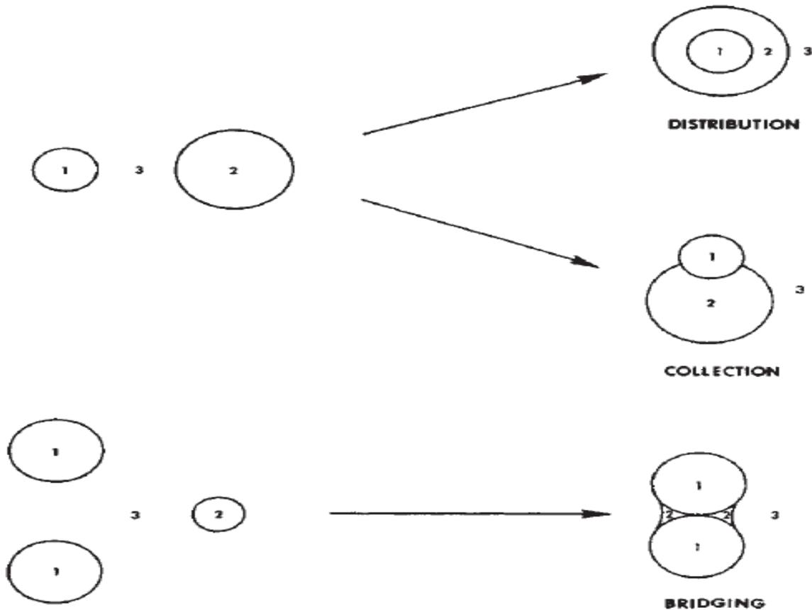
Regimes of separation in a liquid-solid-liquid system. Phase 1 = Particle; Phase 2 = Liquid (dispersed); Phase 3 = liquid (Continuous)
